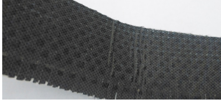
Figure 4.30: Fibre-tow buckling of a [(0/90F)_8] elastomeric laminate.
