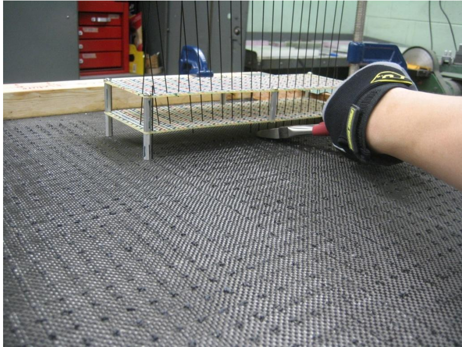
Figure 31. Fabricator cutting carbon pultruded rod
