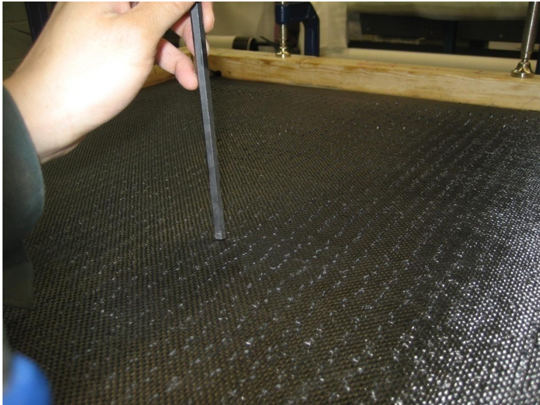
Figure 36. Pins being pushed further into the core to ensure smooth surface
