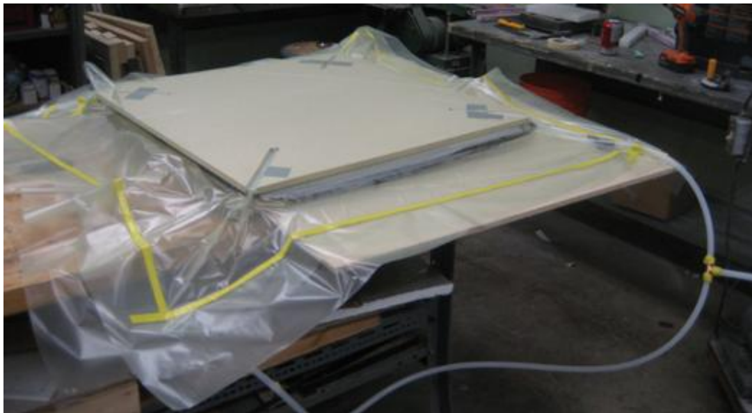
Figure 37. Vacuum bagging of the TCS panel
