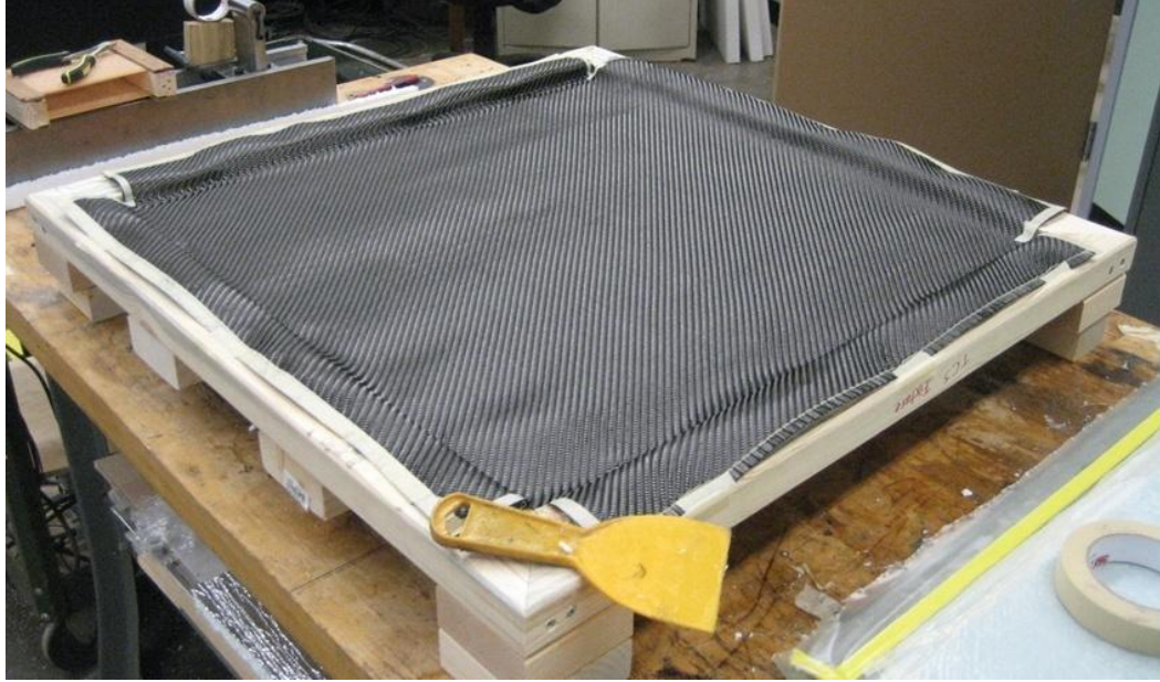
Figure 32. TCS panel fixture – showing the bottom carbon fibre sheet lay-up
