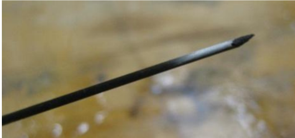
Figure 35. Carbon pultruded rod is trimmed to improve penetration performance
