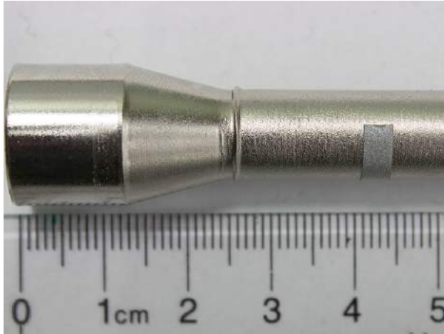
Figure 8.5: A failed specimen showing an axisymmetric buckle fold near the neck region of the specimen. This is an undesirable failure location and indicative of high stresses in the neck region.
