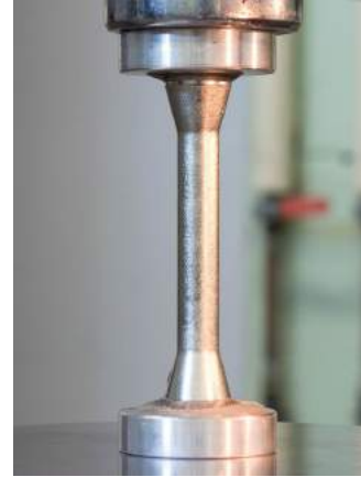
Figure 8.4: A dogbone sample mounted in aluminium collars prior to test. Note the weight on top to keep the sample pressed down as epoxy cures
