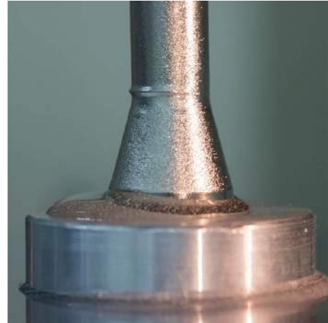
Figure 8.6: A failed specimen showing a non-axisymmetric buckle fold near the neck region of the specimen.
