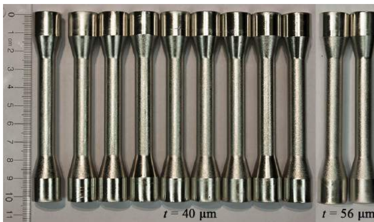
Figure 8.2: An image of all 11 samples as received from Integran with given nanocrystalline metal coating thickness t as indicated. The samples were coated all around with metal, including the top and bottom ends of the geometry.
